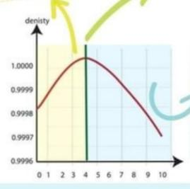
when the temperature rises above 4°C the Water expands as it gains heat energy so the molecules move rapidly and the distance between them and volume increase so its density decreases.
