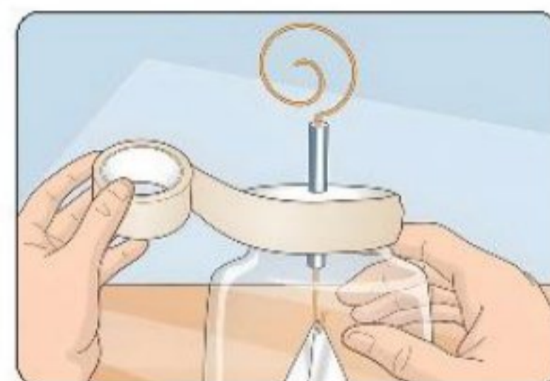
Figure (27) (9) Fix the cap tightly on the glass bottle with duct tape
