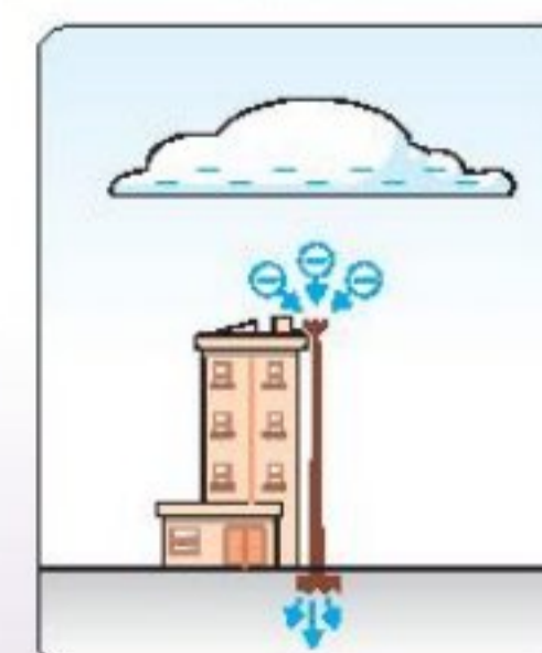
Figure (12) Lightning Rod
