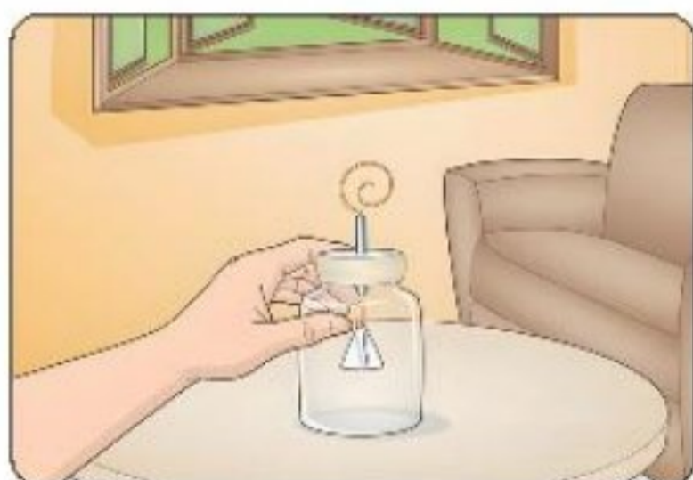
Figure (28) (10) Place the electroscope model in a dry, non-humid place
