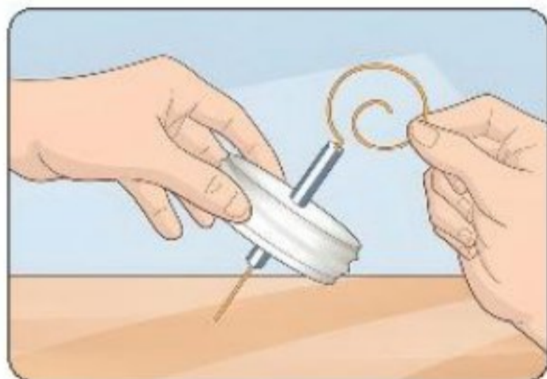
Figure (22) (4) Insert the copper wire into the juice straw
